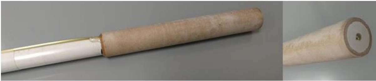
Figure 13: Second dummy sting with cavity pressure tap.
